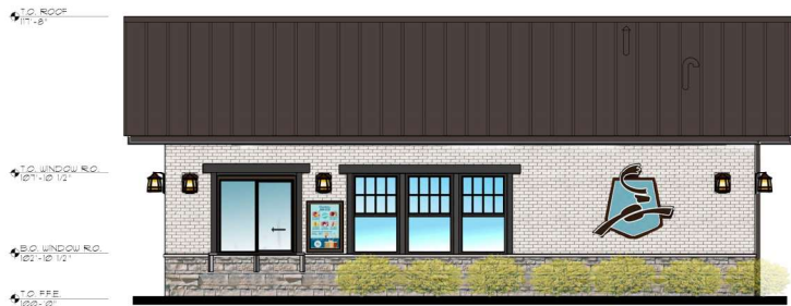
1 SIDE ELEVATION (SOUTH) - PRIMARY FACADE 1/4" = 1'-0"
