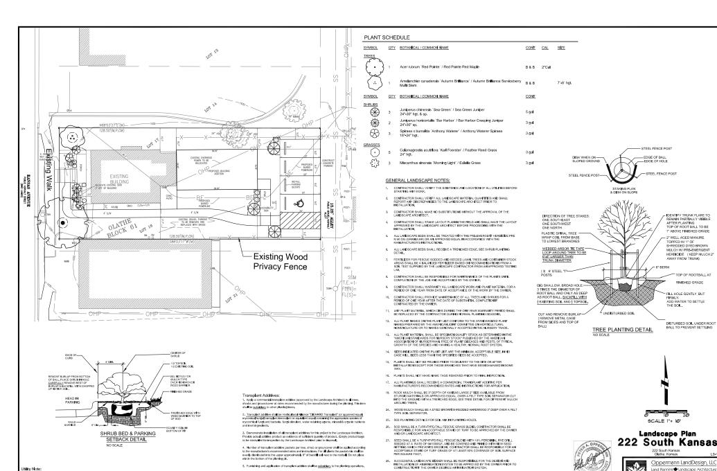
Utilities shown on plan are diagramatic and some may be missing, Before starting any construction call appropriate locating service, in Kansas call 1-800-DIG-SAFE (344-7233) to have utilities located.
