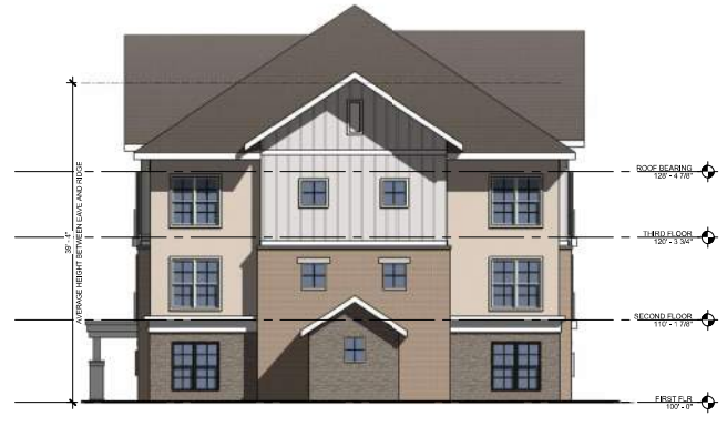
3 BUILDING 4 - SIDE ELEVATION - 2 PR4.5 1/8" = 1'-0"
