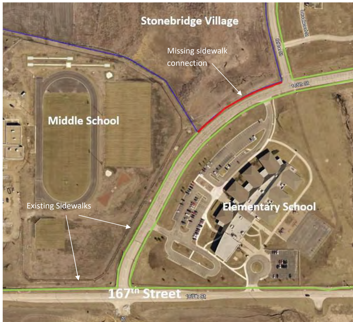
View of subject property, existing sidewalks (green) and the missing sidewalk link (red)
