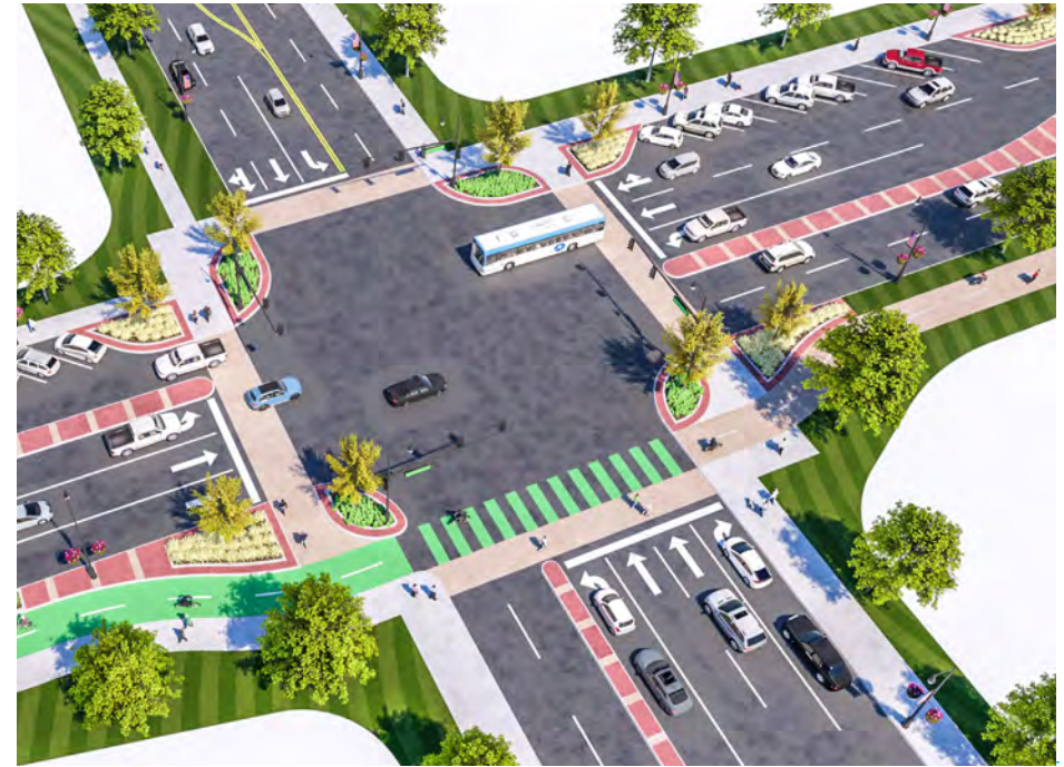
Protected intersection concept for Kansas and Santa Fe. Kansas cycle track at left crosses Santa Fe and transitions to a shared use path along the Courthouse site.
