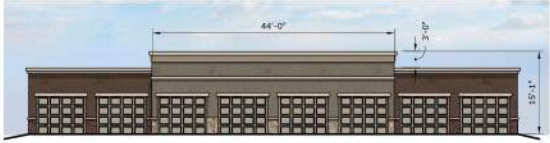
ELEVATION FREE STANDING GARAGE SCALE: 3/32" = 1'-0"
