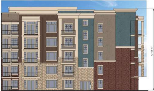
ELEVATION 5-STORY MULTI-FAMILY BUILDING SCALE: 3/32" = 1'-0"
